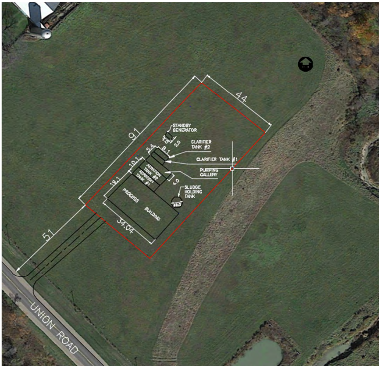
Figure 2-1: Shedden Location – Extended Aeration Facility
