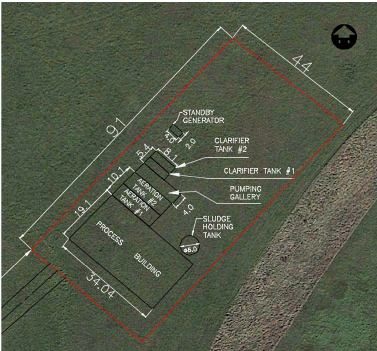
Figure 2-2: Shedden Location – Extended Aeration Facility Detail
