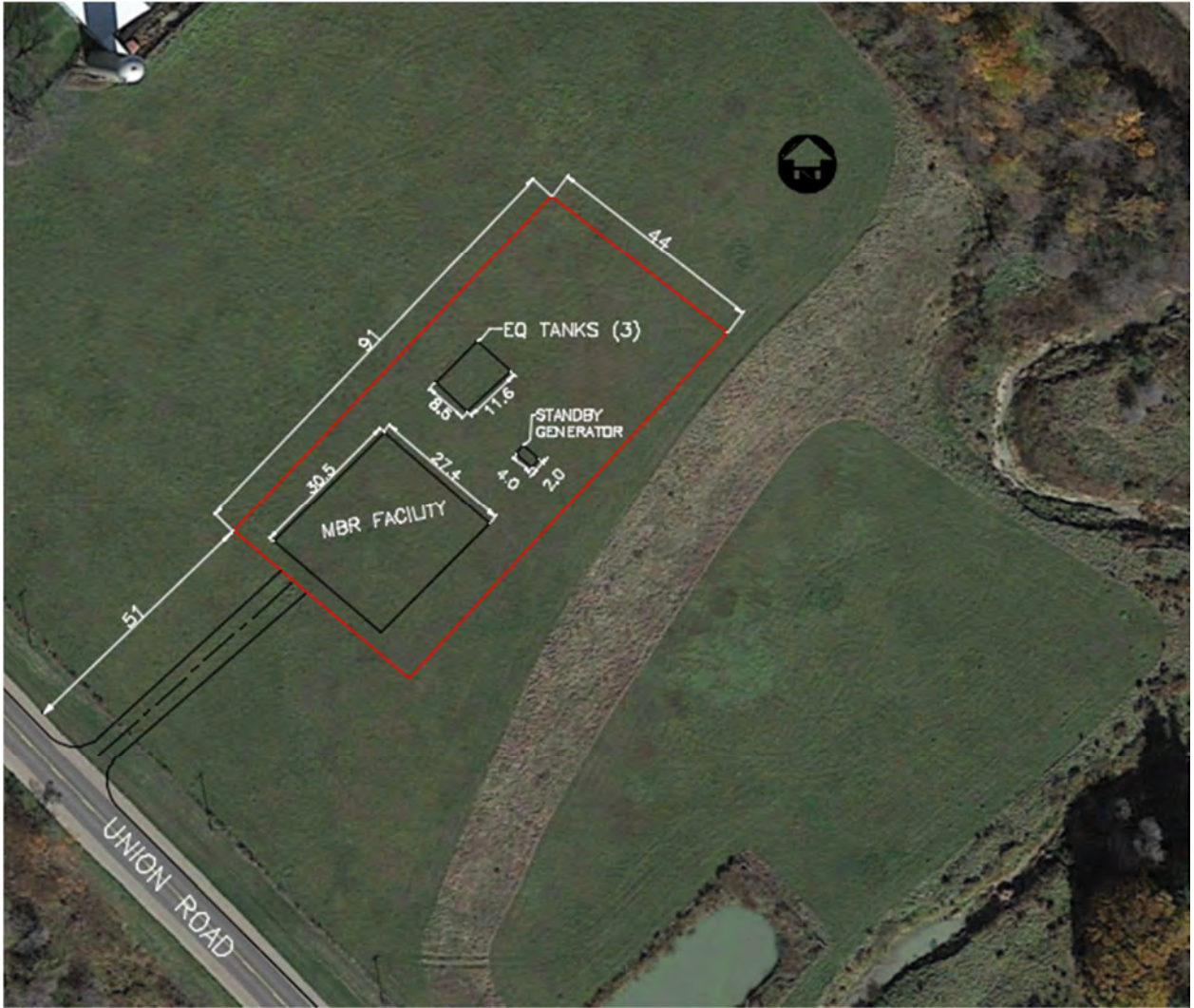
Figure 2-5: Shedden Location – MBR Facility
