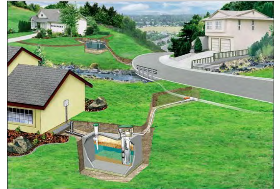
Example of a STEP Low Pressure Sewer
