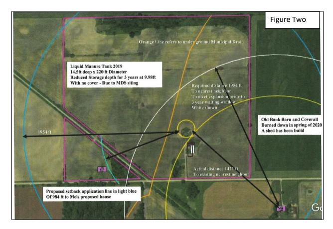
The proposed expansion to the existing manure storage facility (pit) is located 433 metres (1421 feet) from the dwelling at 35507 Fourth Line and 300 metres (984 feet) from proposed dwelling at 35246 Fourth Line.
