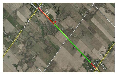
**Figure 1 –** Sanitary Sewer EA Routing (red – sewer, red square – WWTP, green – forcemain)
